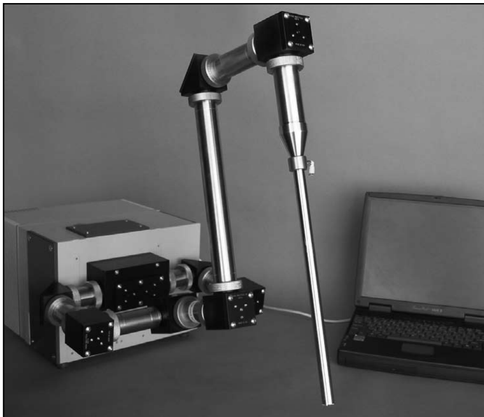
Figure 2: DMD-270 Diamond ATR Probe coupled to a Bruker IR Cube FTIR spectrometer by means of a custom Axiot interface.
