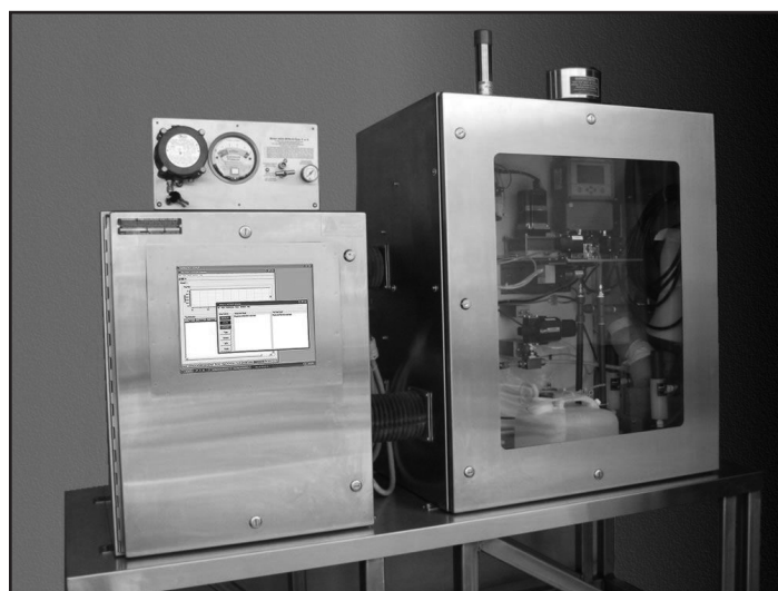
Figure 4. A fully automatic Sparging-IR system for 24/7 on-line operation.
